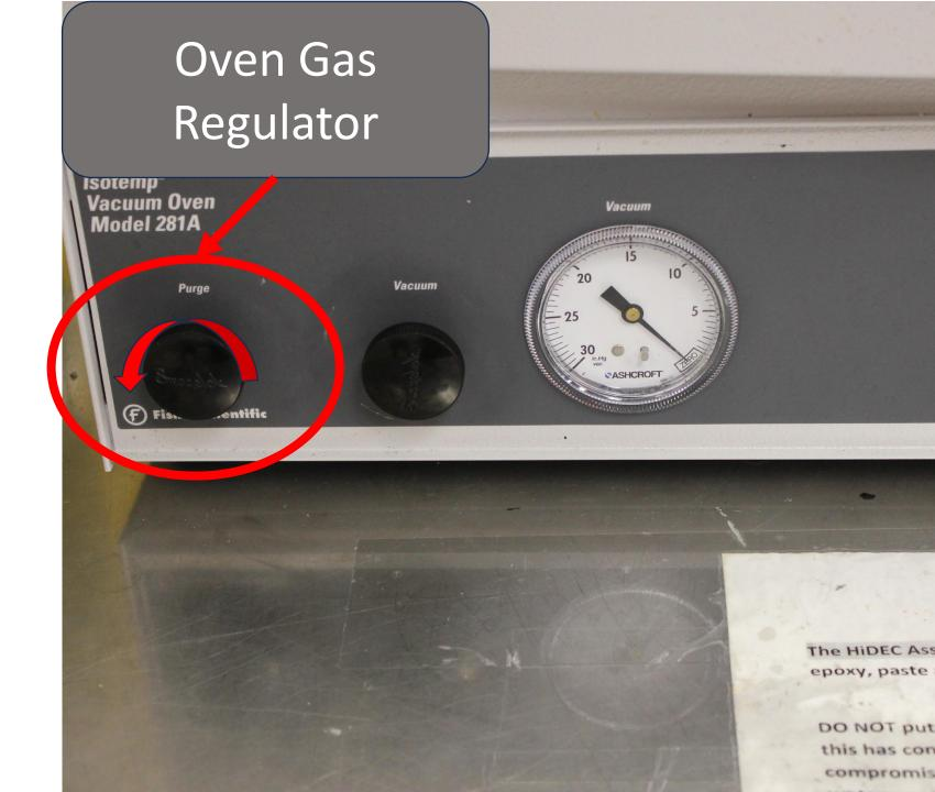
When finished retrieving your parts, turn the purge and vacuum regulators clockwise until they stop to shut off gas and vacuum suction to the oven.
