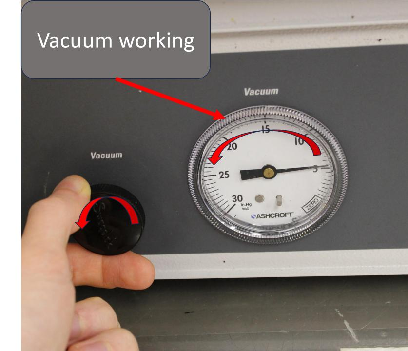
It will take about ~1 hour to fully pump the chamber down. Perhaps longer depending on your sample composition and the cleanliness of the oven.
