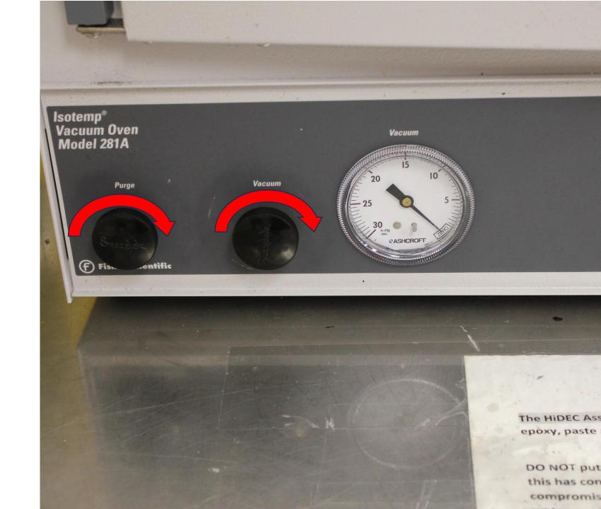
When finished retrieving your parts, and shutting off gas and vacuum to the oven, return to the primary gas control valve, and return it to the off state.
