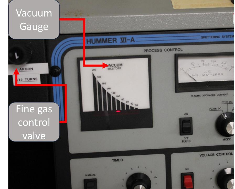
Identification Once the fine gas control valve is completely closed, IE not leaking expensive argon. You may hit the main power switch to shut off the vacuum pump and sputterer.
