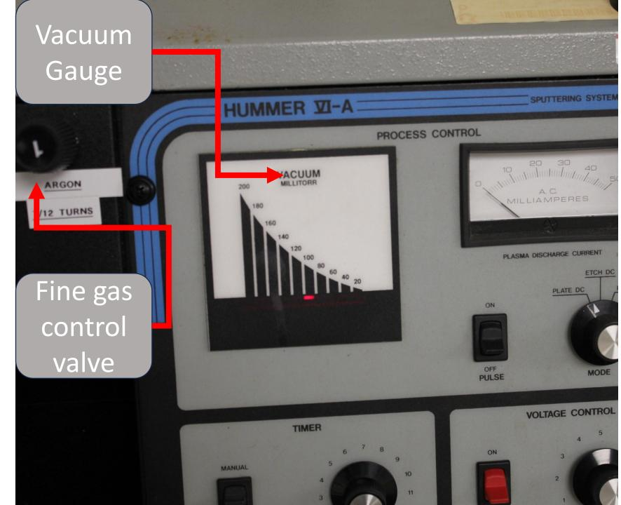
Identification Once the purge is complete, set the fine gas control valve to a position such that the vacuum pressure reads either 40, 60 or 80 **millitorr.** The exact gas pressure will change the deposition rate. You will have to determine the exact value you require for your own research. **Or consult with HiDEC** staff if this range wont work.
