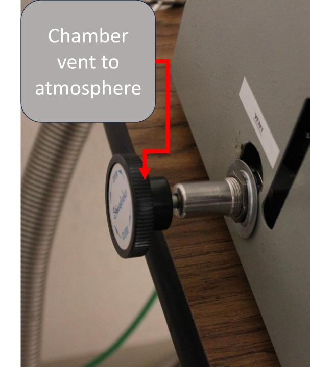
Once the vent valve is closed you can insert your samples into the chamber and close the lid on the sputterer. The lid may require some gentle maneuvering to seal properly. You will only know if it is properly sealed by listening until the humming is damped by the closure of the silicone gasket.
