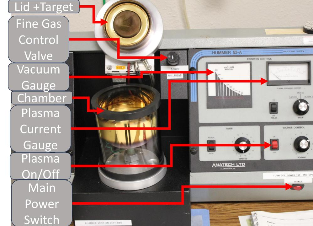
Identification Look at the color of the metal on the chamber wall. It should match the color of the installed target. Your samples can be placed on the sample stage.
