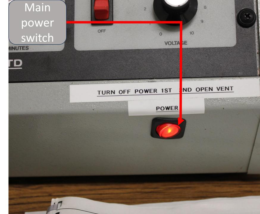
Once the high voltage, main power switch and vacuum pump(from the main power switch) is turned off and the fine gas control valve is closed completely you may open the atmospheric vent on the left side of the machine to return the chamber to atmospheric pressure. You will hear this as an audible hiss of relief as the air rushes back into the chamber
