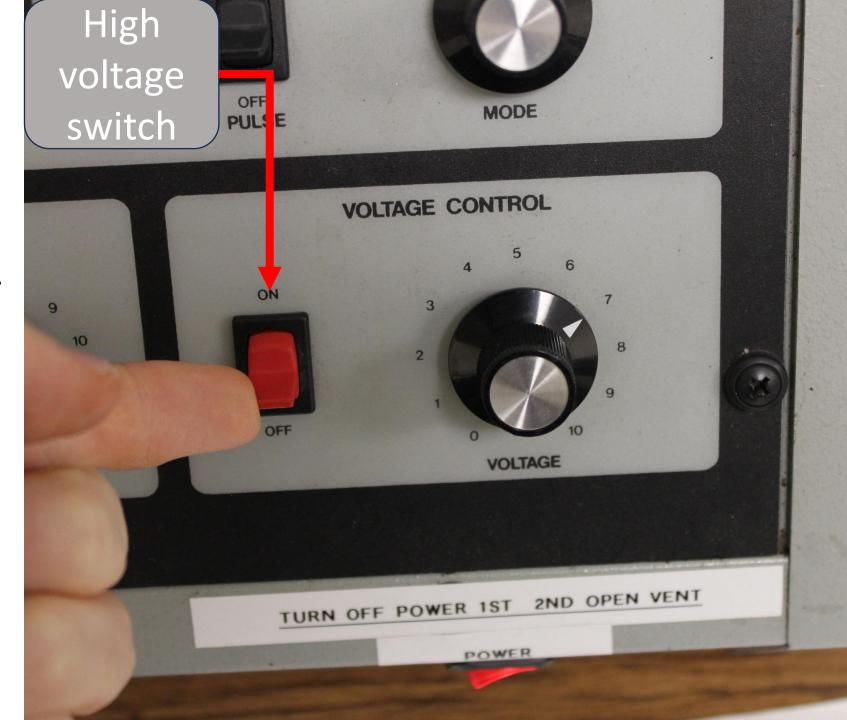
Identification When you activate the high voltage at the correct pressure you should hear a click and a low buzzing sound, and see a steady and somewhat dim purple glow from the chamber. It may be blocked from view by the metal sputtered on the chamber walls.
