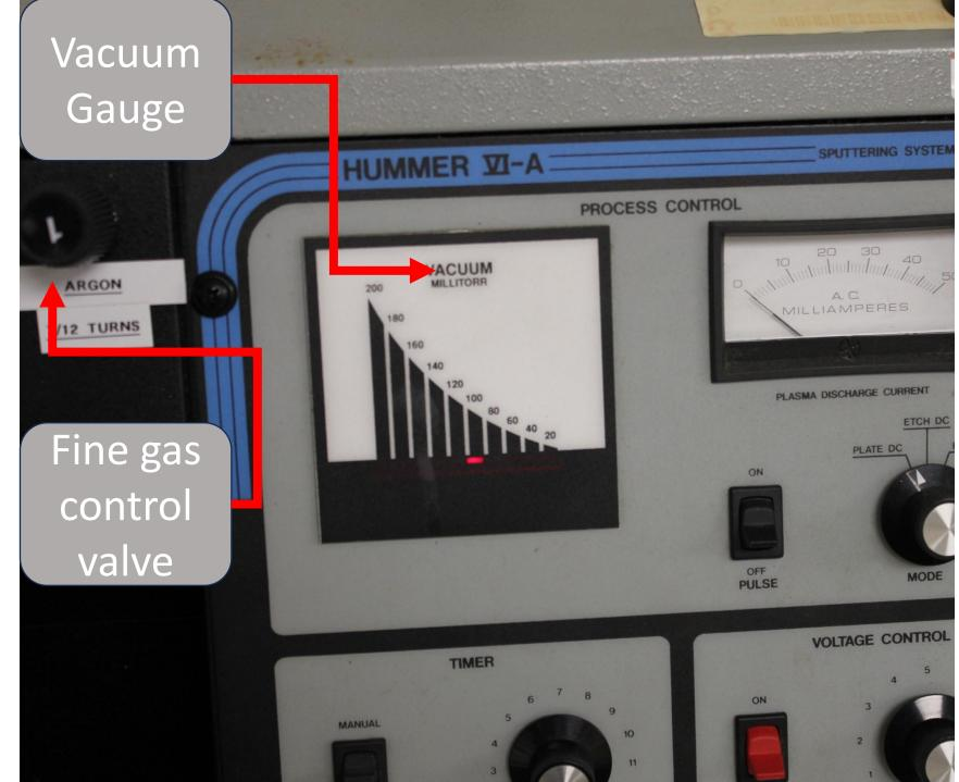
Identification Turn the fine gas control valve counter clockwise until the pressure reaches 200 millitorr. Then turn the fine gas control valve clockwise until the chamber pressure returns to 40 millitorr.
