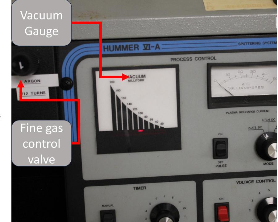
Identification Once the chamber is purged and at pressure, you may switch the dc high voltage source on, by flipping the big (non lighted) red switch under "voltage control" on the front panel of the machine.
