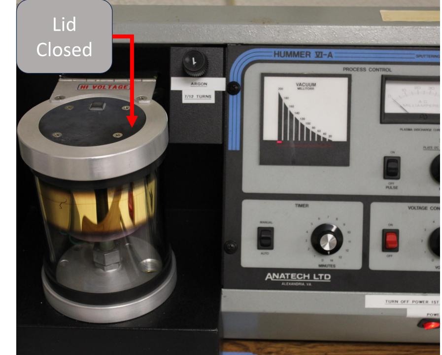
Once you get a good seal on the lid and chamber, you should check that the voltage setting is about 7-8 KV, and the mode is set to "DC plate".
