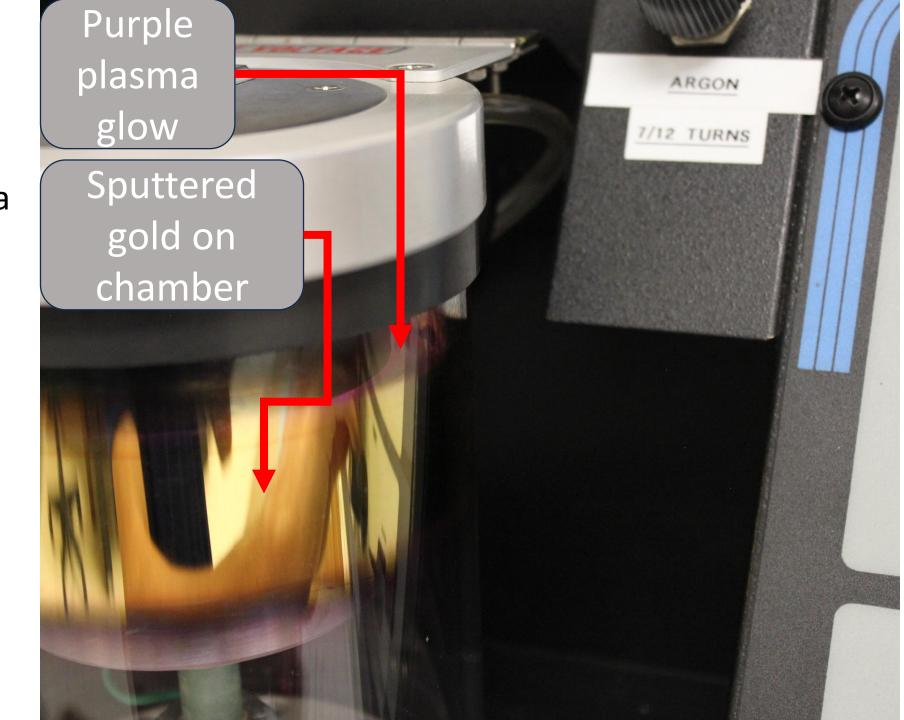
Identification When you have finished depositing for your desired time (no more than 5-10 minutes) you may switch off the plasma. By turning the red high voltage switch off.
