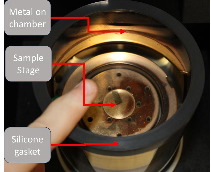
Deposition works on "plate dc" setting Deposition can be performed in pulses or continuously.
